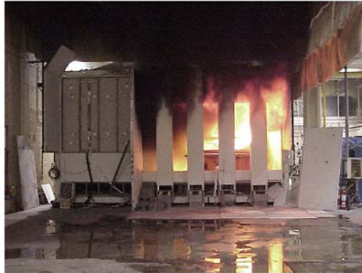
Figure 4-6. Multiple workstation fire experiment.
