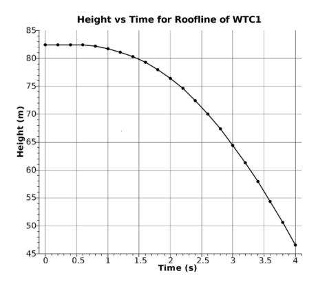
Figure 1: Graph of the height of the roof line (measured from an arbitrary origin) vs. time at 0.2 second intervals. Note that once it begins to fall the path appears approximately parabolic.
